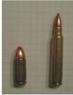
Figure 6 Comparison of a 9×19 mm NATO (left) to a 5.56×45 mm NATO (right) cartridge.
